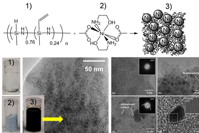
Fig. 1. The formation of Ni-polysilazane precursors (3) by reacting of polysilazane polymer (1) with Ni-complex single crystal (2). TEM shows the produced Ni/SiCNO nanocomposite by thermolysis at 700 °C
